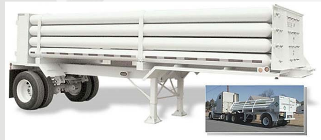
Example of a Tube Trailer for transporting 99.999% Helium Gas at ~4,000 psi
