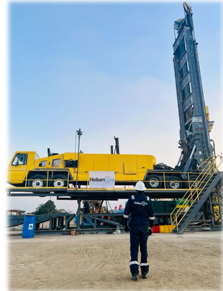
Epiroc Predator 220 drilling rig rigged up at Tai-C wellsite, Rukwa Basin
