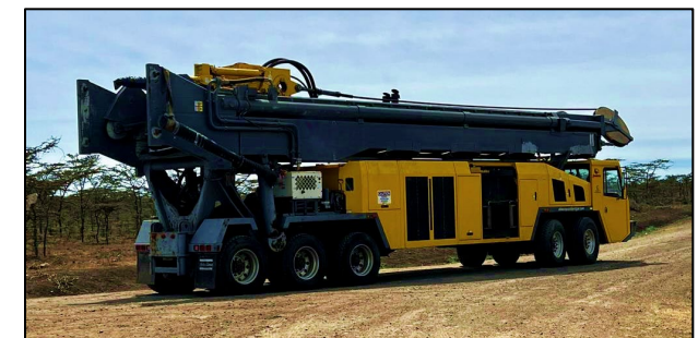
Truck mounted Epiroc Predator 220 drilling rig
