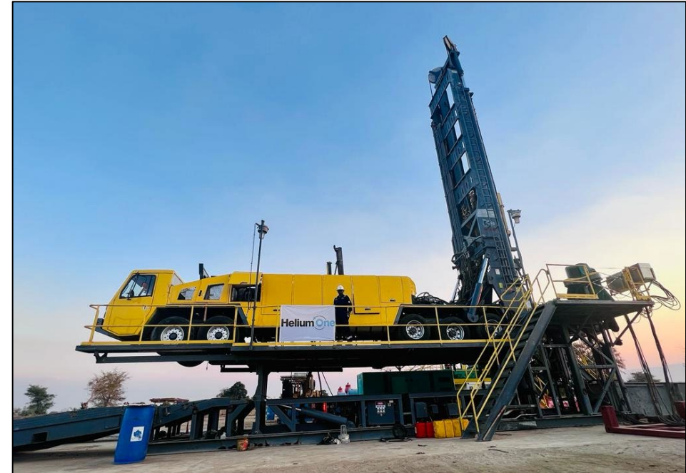
Epiroc Predator 220 drilling rig rigged up at Tai-C wellsite, Rukwa Basin
