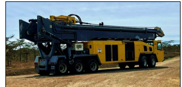
Truck mounted Epiroc Predator 220 drilling rig
