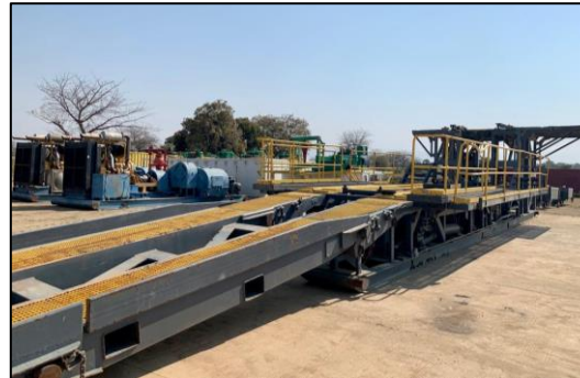
Assembly of rig substructure Tai-C well site
