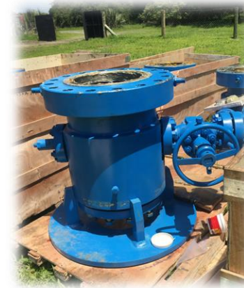
13 5/8" 'A' section of wellhead for Tai-C at Rukwa site
